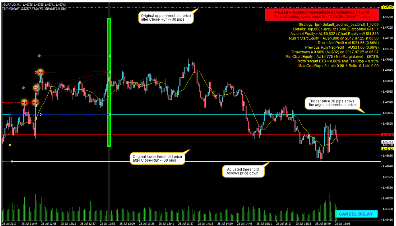
Figure #5: This image illustrates a strategy where Auto Restart After Profit = After-Pips-Retrace , Restart Seconds Delay is zero, Restart Pips Up or Down = 30, and Restart Pips Retrace = 20. The lower threshold was hit first, and it follows the price downwards. The cyan-colored line indicates that the trigger has been activated, and it continually adjusts to be 20 pips above the threshold. When the price moves back up to the trigger price, ForexGM becomes active and the next Run commences. If it is required to continue trading before the price reaches the trigger level, press the Cancel Delay button and the next Run will start immediately.
