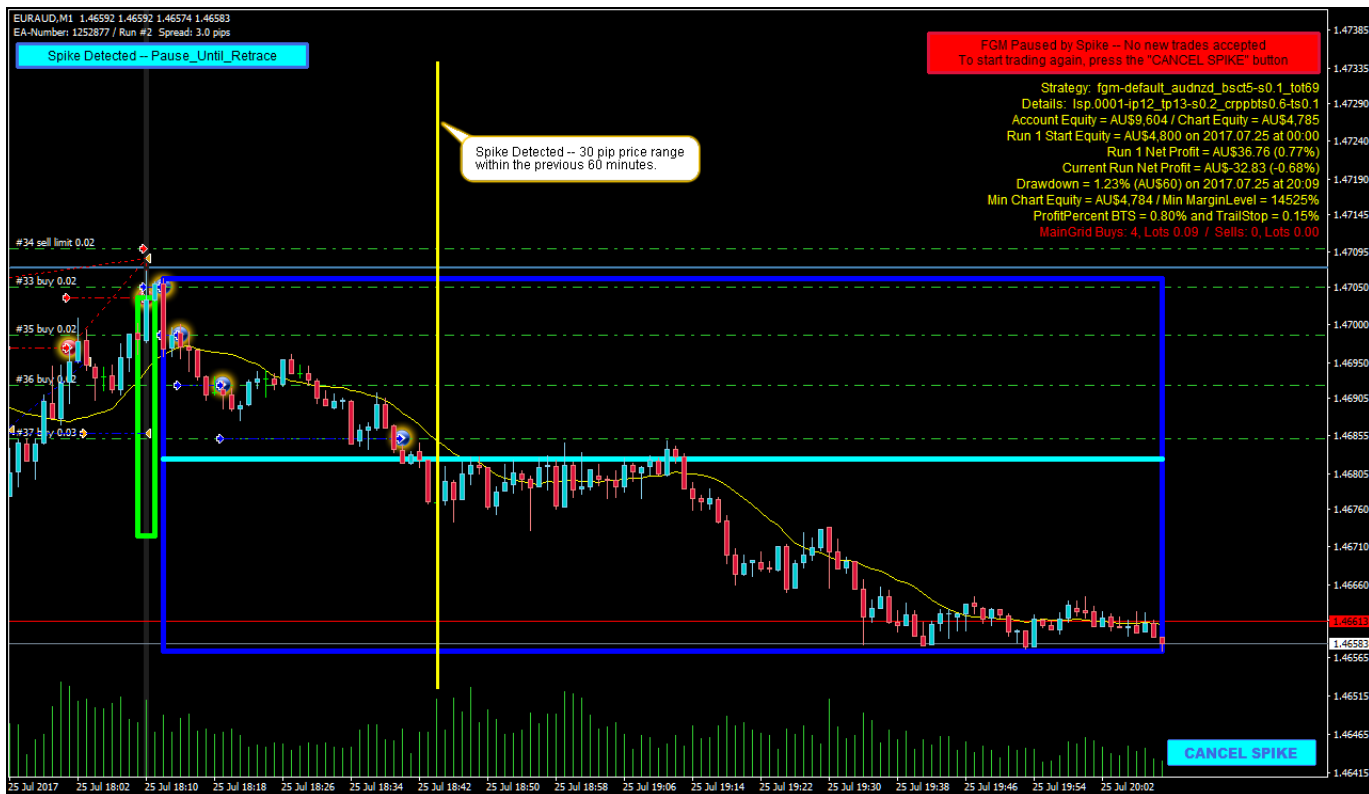
Figure #4: This image illustrates a strategy that has spike detection set for a 30 pip range in a 60 minute window, Spike Option = Pause Until Retrace and FSpike Pause Retrace Pips = 25 . The left side of the dark-blue rectangle indicates where spike detection started, and the cyan line shows the retrace price that will cancel the Pause. The vertical yellow line has been added to show the time the actual spike was detected. Normally this point would be 60 minutes after the start of the monitoring interval, but because a Stop-Run occurred within the previous 60 minutes, the Stop-Run time becomes the temporary start of the monitoring interval. In this case, the spike is downwards, and the retrace price is 25 pips above the minimum price since the spike occurred. Notice that absence of grid-lines after the spike is detected. As with other Spike Options, this Pause can be cancelled by pressing the Cancel Spike button.
